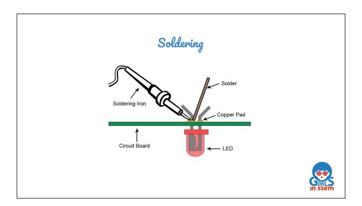
For the woven speaker, the additional technique you will need is soldering when connecting the wires to the amplifier chip.
