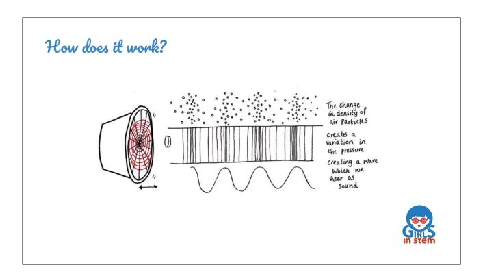
The sound waves are created, due to the up and down movement of the speakers face.
