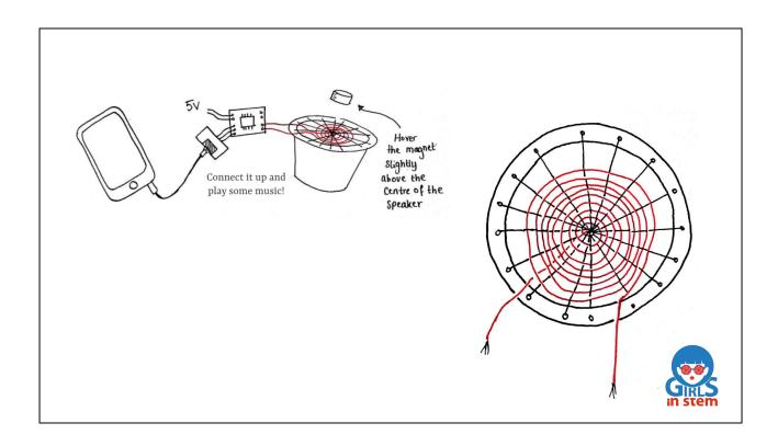
This illustration shows how the coils for the electromagnet are formed using a spider web of the thread in a yoghurt pot.
