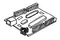
Arduino is an open-source hardware and software. The hardware is a board with a microcontroller, as shown in the illustration. It can take an input (such as a signal from a sensor) and create an output (such as make a motor turn or an LED flash). The board works with Arduino IDE software, which allows you to create the code that controls your board, the inputs it reads and the outputs it creates.
