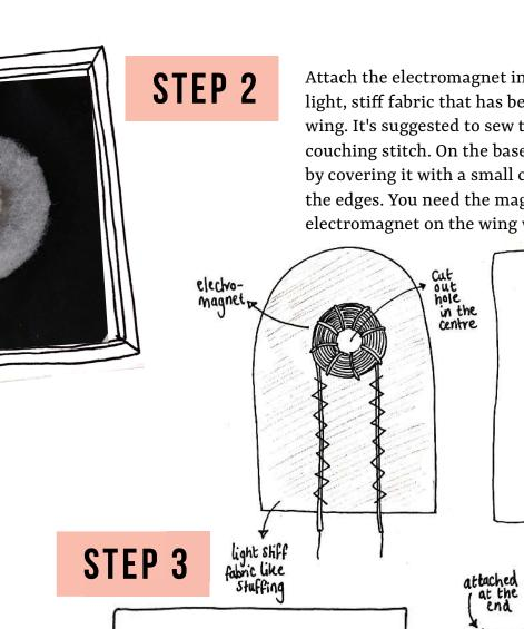
Attach the electromagnet into position on the wadding or light, stiff fabric that has been cut out into the shape for the wing. It's suggested to sew the the legs down using a zig zag or couching stitch. On the base fabric, sew the magnet into positon by covering it with a small circle of fabric and sewing around the edges. You need the magnet to line up with where the electromagnet on the wing will sit.
