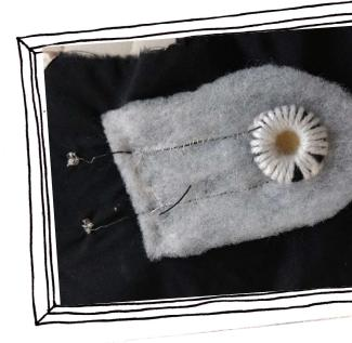
Make a wing that can flap up and down when an electrical current is applied. The flapping wing uses electromagnetism to create movement in a similar way to the flip dot eye.
