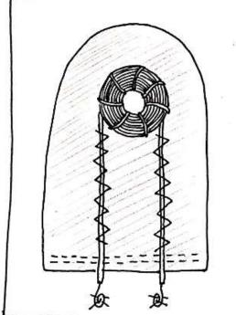
magnet centred to Attach the wing to the base the middle hole fabric piece by sewing along of the electrothe bottom edge with a running stitch. Make sure the electromganet is well positioned over the magnet like shown in the image above.
