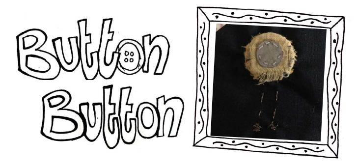
The Button Button is another two-state (on and off) button made from textiles. It uses a plastic button, sewn in position with conductive thread, which than can be integrated into a circuit.
