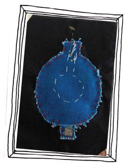
The fabric button is a simple two-state button which is made from textiles. It has two connecting points (positive and negative) which allows it to be integrated into a circuit.
